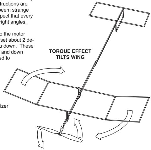
The reason for wanting the wing to fly level is that a wing will generate lift in a direction perpendicular to its path of flight. If the wing is banked, the lift will be directed at some angle less than the desired vertical and increased energy will be required from the motor for the airplane to gain altitude.
