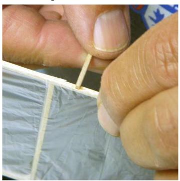
Glue the 6.5 cm wing post to the back of the TE at the 1-cm mark you have made. The angle of the wing post should be slightly skewed to the left when viewed from behind the TE. Skewing the wing posts will translate into the desired twist in the wing when they are inserted into the sockets. (Review the part about Circular Flight earlier in this
