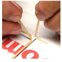
of the wing and all four corners of the stabilizer with paper gussets. Next place gussets at the wing center rib where it meets the LE and TE. There are no gussets at the other two ribs.
