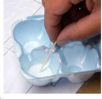
Use a scrap of the Styrofoam to transfer the cement from the can to the egg well so that the
