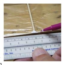
wing post to the front of the LE at the mark. Make sure that the angle of the wing post on the LE is at 90 degrees to the LE.
