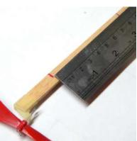
With a sharp razor blade cut a V-shaped grooves in the motor stick at the two marks from the top of the motor stick to its bottom. The groove should be less than 1 mm deep.
