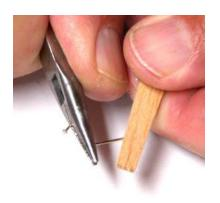
Make a second bend in the long leg at right angles away from the dip in the J.
