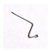
Coat it with glue at the motor stick to keep it from twisting. The propeller assembly is pushed onto the front of the motor stick so its thrust hook and the rear hook are on the same edge.
