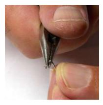
Push the sharp point into the rear of the motor stick with the open end of the dip facing towards the rear of the motor stick.
