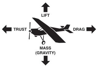
Many of you have probably seen the standard diagram of the aerodynamic effects of the four parameters: **Lift, Thrust, Drag and Mass.**Good airplanes have Lift and Thrust emphasized with Drag and Mass minimized. We shall try to show how these effects can be better understood to make your airplane fly or make your airplane fly better.
