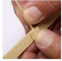
is re-assembled, the same relationship results. A second, equally important, outcome of using the socket and dowel connection is that the proper warps can be established for flying the airplane in a circular pattern. The word "warp" may sound like a bad thing for a wing and excessive warps are bad. The warps are actually given names like "Washin" and "Washout" because they help the airplane stay level in circular flight. See the section to about asymmetric construction and circular flight later.
