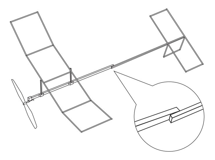
Glue the tailboom assembly of the stabilizer and fin to rear of the motor stick, overlapping about one centimeter. The tailboom should be attached so that it slopes up a few degrees, no more. This will provide the necessary angular difference between the wing and stabilizer.
