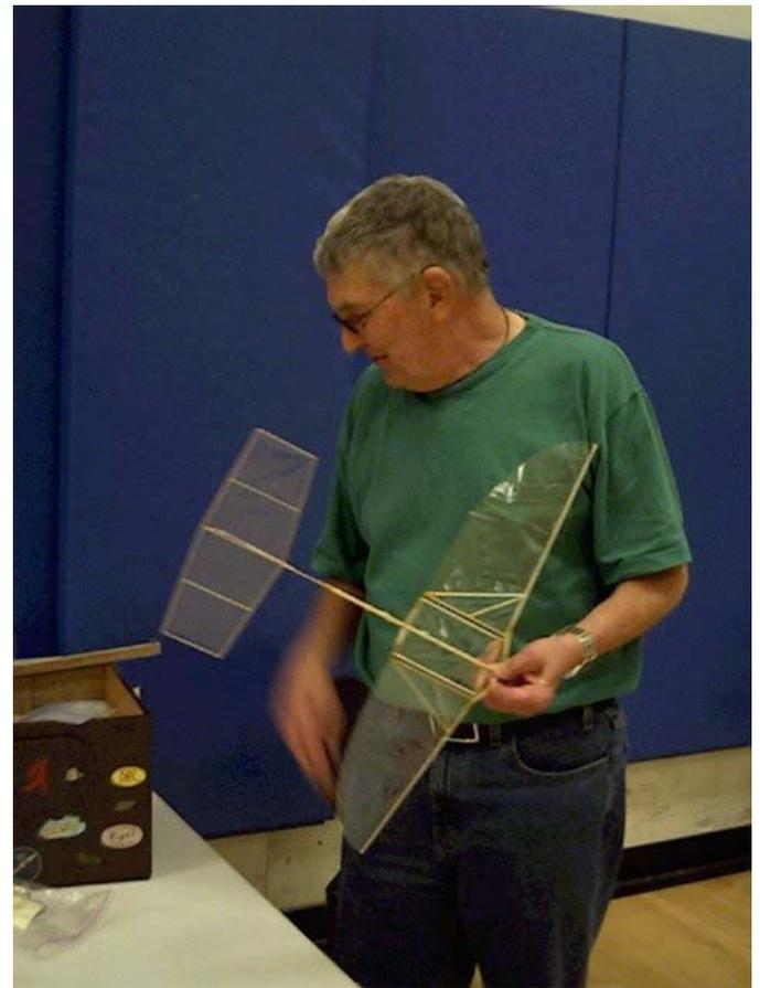
Henry Smith had an ornithopter. It is powered by a twisted rubber band that turns a crank that flaps the wings up and down. It is an inefficient propulsion system, so the motor must put out a lot of torque and the fuselage must be pretty stiff and heavy. It is amazing to see these things fly..
