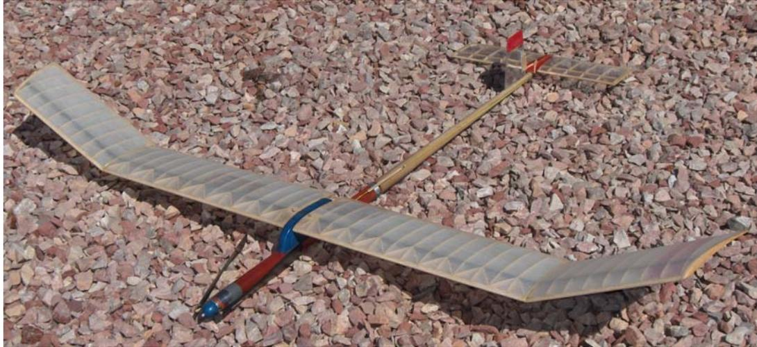
Thanks to a generous donation by Dick Strang, the Magnificent Mountain Men has this Super Candy G F1G to raffle. The model is the basic Andrey Burdov model marketed by Starlink. It has been flown and there is a small repair to the covering on the LE of the stab. It has a fiberglass body and pylon, carbon spar wing and is equipped with a button DT timer.
