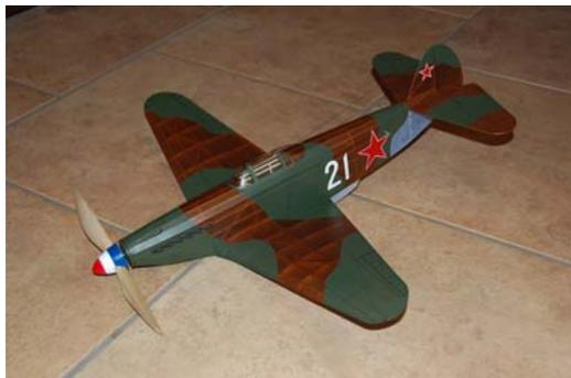
35 grams balanced (no nose weight required); 18 gram motor and 9.5" carved paulownia prop; 104 square inches. Detachable wing and radiator via rare earth magnets; rotating stab DT; button timer.
