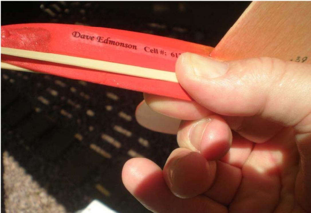
Typical launch grip. Fuselage rests between thumb and index finger underneath wing. Thumb and index finger retain the rubber at the attachment point. Make sure you put your name and telephone number on your model. Occasionally you get called when one is found. It is always interesting to find out where the model landed on one of those contest winning fly-away flights.
