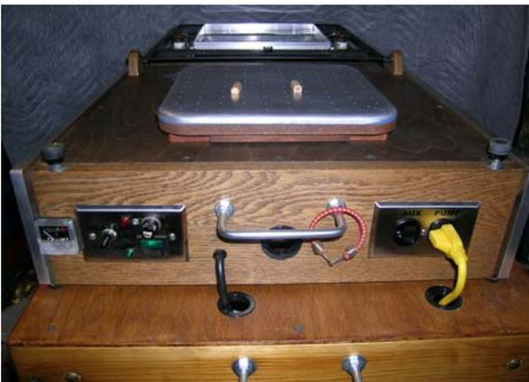
Two meters show input power and actual vacuum. The side view shows two master molds for the Walston. You can see the flat side on the table.
