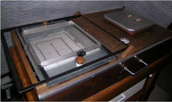
On the left is the film carrier with the heating coils and on the right is the vacuum table with all the holes to pull the high vacuum. The heated film is quickly lowered over the master forms and then the pump is started to pull it down instantly.
