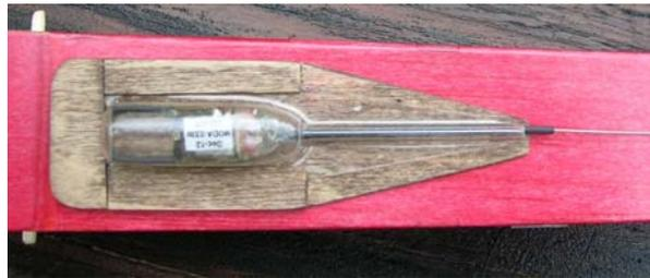
This photo shows the slide in holder I made for the transmitter bubble. The flanges left after I trim the bubble from the forming sheet are trapped under the 1/32 ply rails. If it needs to be tighter, I just add a slip of paper under the transmitter. The bubble weighs 0.9 g and the 1/32 ply holder is 1.6 g. The antenna is held in place with a few pieces of small straw tubing along the top of the fuselage.
