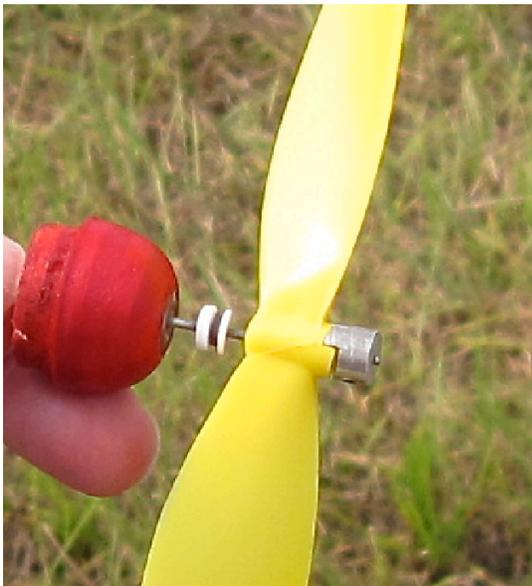
One important thing to remember — file a small flat spot in the prop shaft where the lock screw is to contact it. Otherwise, there's a high probability you'll hear some exciting noises as the drive disappears and the wound motor goes wild. Ask me how I know!!
