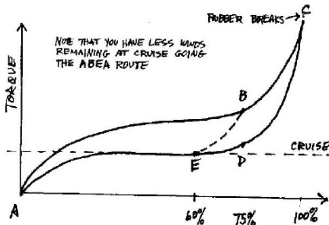
The graph A-B-E-A is what things look like when you don't wind to near max. So when you wind to B and launch there is still a big torque burst before the torque drops to a cruise level around E. Notice that by taking the A-B-C-D route you arrive at a more comfortable level with a lot more winds. So, actually, it is better to walk down the block and turn around and come back.
