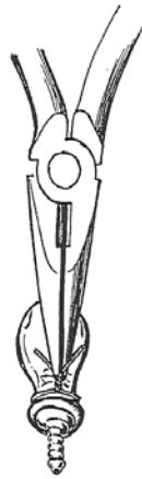
Grab the wires where they cross and twist until snug. (too loose and it leaks, too tight and the wire breaks)
