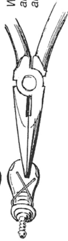
Wrap the binding wire around near the lip and cross the ends
