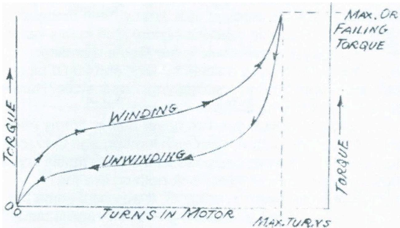
Using the RTM was a real eye opener emphasizing the interplay of torque and tension. The ideal "S" shaped hysteresis loop of the typical rubber motor being wound and unwound like that shown below from McCombs is hard to reproduce in the real world.
