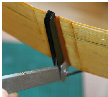
These photos show the strong CF and ply wing saddle and the wire spring to pop the wing up. By the way, it's a Sweep 30 inch TLG, designed by the late great Lee Hines.
