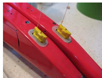
A Benns' Bowler and Edge Brim ensures the AliLoc Tx is clear of a conducting fuselage
