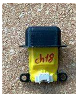
A Benns' Bowler and Edge Brim ensures the AliLoc Tx is clear of a conducting fuselage
