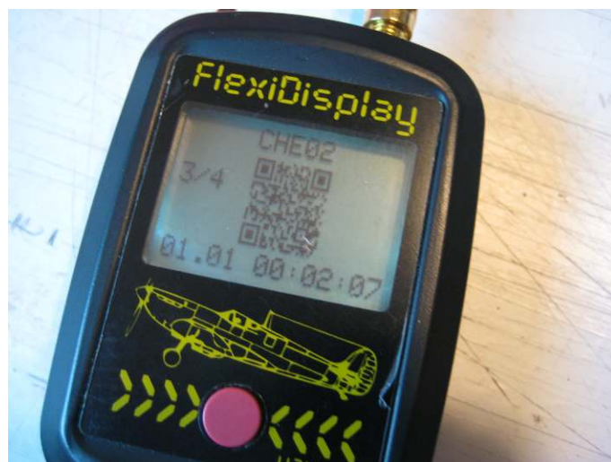
The QR Code Screen 3 can now be used to select a beacon for tracking
