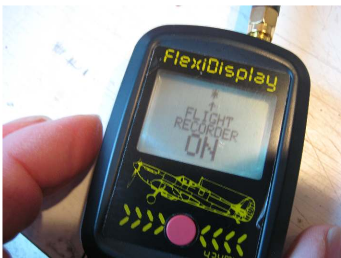
Flight Data is now recorded by pressing the Edge Button for two seconds
