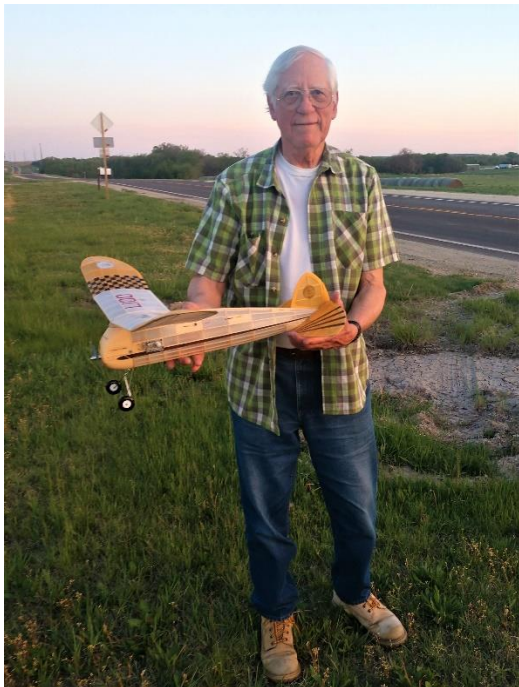
Bill with the Pacer – a Sal Taibi model with a TD-020 for power in it. The hole in the nose is for priming
