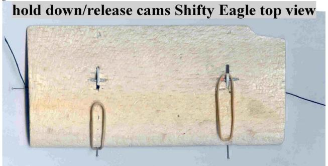
I hate the idea of having all this crap protruding from the wing, but in any case I have to have template fences mounted above and below the wing chord that determine the climb and glide settings. So, the cams are virtually hidden...though I imagine the templates will cause a major disruption in the airstrip. Oh, well...nothing is perfect. I guess a better way could be found, but I don't know if I could design it much less construct it.
