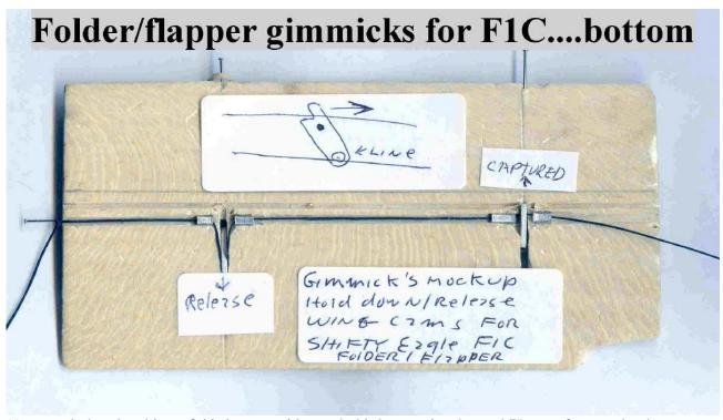
(As a reminder: the object of this is to provide two hold-down points located 7" apart from each other as centered in the 22" inner wing panel (s). A rubber band from each cam goes around the folded wing to not only hold it in the folded position but to compress the symmetrical airfoil formed naturally as an un-squeezed 20+% section down to a low drag version of 13%)
