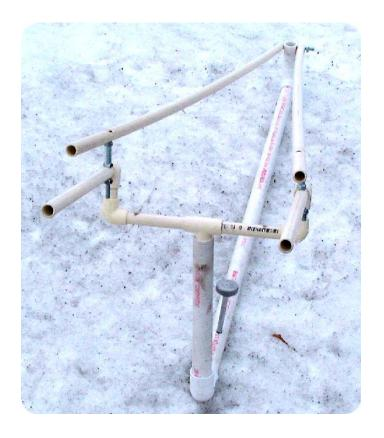
The main ground support is ¾" diameter, the front upright is 12" from ground to top, and the rear tube is 3 ½" from ground to top. The distance between the center of the front tube and the rear tube is 36". The T on the bottom cradle piece just slips into the ¾" tube and there is a 6" piece extending down. I have recessed the screw heads in the top tube so nothing extends above the top tubes so the stabilizer has no obstructions.
