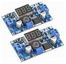
The motor will run just fine on 6 volts but the significant increase in speed makes for tiny bubbles which I did not like plus it burns through solution even faster so I ordered a "HiLetGo LM2596". This handy circuit works as a volt meter but also includes a voltage trimmer which allows me to fine tune my motor speed by turning back voltage to around 4v.
