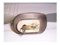
Thrust adjustments are usually made by adding shims behind the nose block. On a visit to Pat Tritle's shop I spotted this nose block. On the front is a small piece of brass drilled to fit the prop shaft. The rear of the block has a large hole to allow the prop shaft to be adjusted to different angles. On the rear there is a blind nut epoxied in place. The brass strip has a hole for the prop shaft and a slot to permit adjustment.
