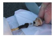
Sometimes a Crocket hook will try to run off to one side of the rear hook on a prop shaft. Roger Edwards uses a piece of heat shrink tubing around the back of the hook and over the front of the rubber motor and this cures the problem for him. I understand a short piece of plastic soda straw works for this too.
