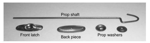
If you are using carved free wheeling props on your O.T. rubber model or FAC model here is a neat freewheel set up from Easy Built models. I use cut off straight pins and slow set epoxy to hold the back piece and front latch to the prop. It works well for me. And Easy Built folks get very high marks for service.
