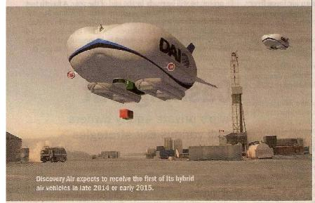
he notion of whether commercial hybrid airships are economically feasible will soon be put to the test. Piggybacking the work U.K. Hybrid Air Vehicles is doing for Northrop Grumman on the long-endurance multi-intelligence vehicle program, Canada's Discovery Air will take a stab at offering commercial services using a 50-metric-ton (110,231-lb.) version. The goal is to provide cargo options, particularly for remote locations
