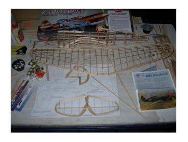
From the work table of John Merrill, a Guillow's P-40 Warwark started. This model will have a wing span of 28" when completed.
