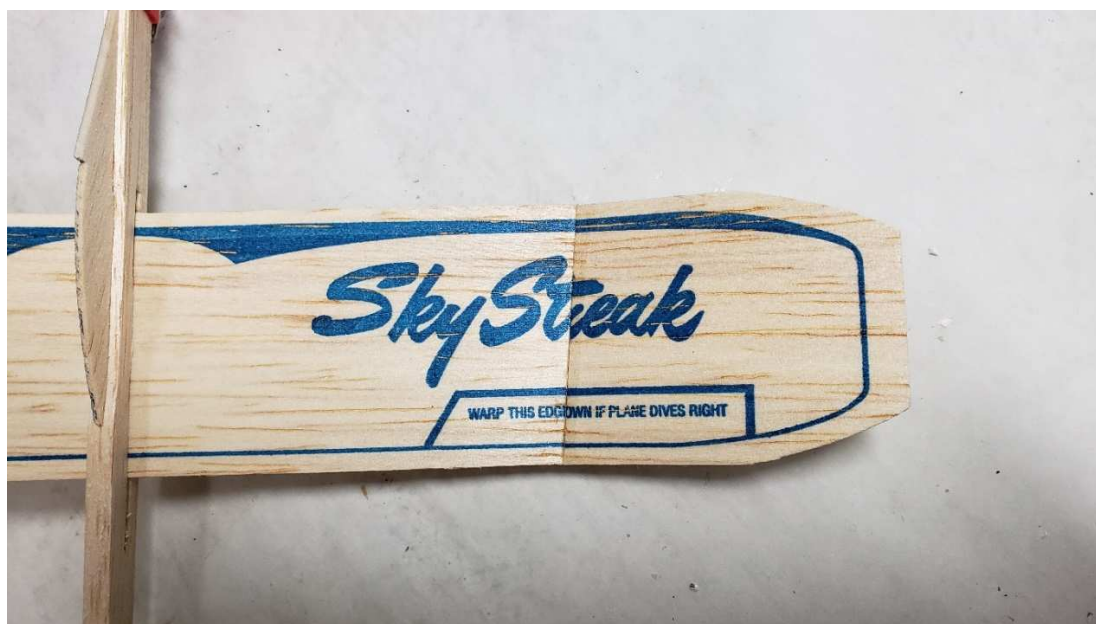
Skewed Wing Tip Section Joint for Increased Dihedral and Washout
