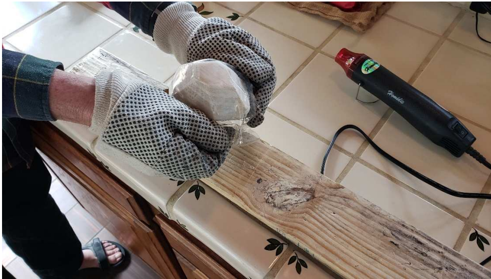
Heat Forming a Plastic Canopy Over a Balsa Wood Mold Plug
