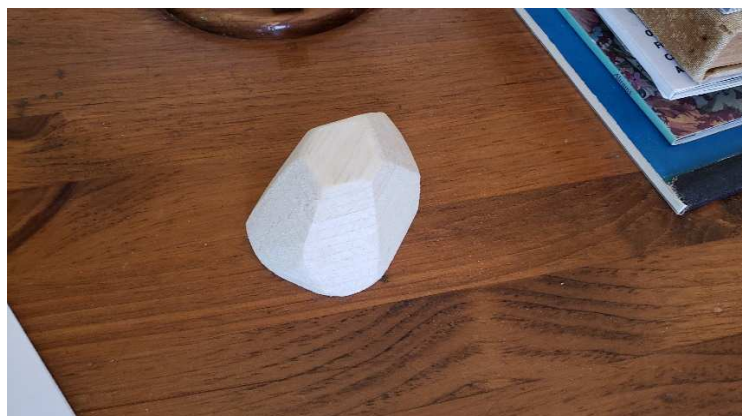
Mold Plug Made from Laminated Balsa Wood Sheet
