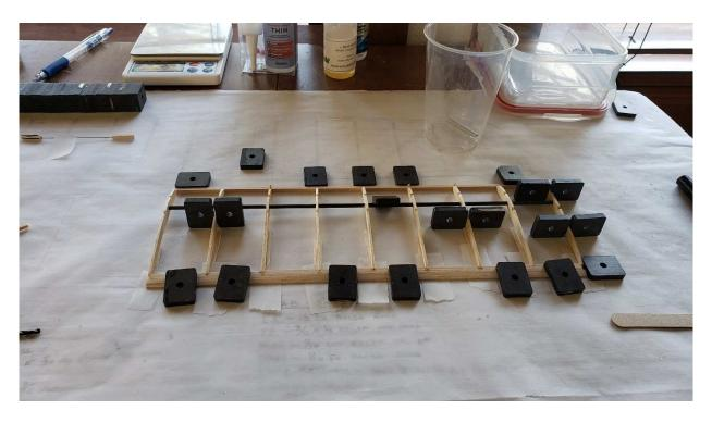
**Rectangular Magnets Holding Wing Ribs Vertical**
