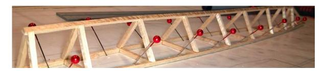
Straight Pins Leaning Against Triangular Stick-Built Balsa Wood Fuselage
