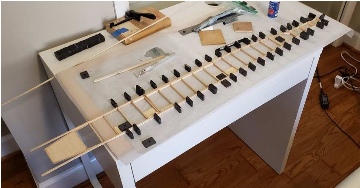
Second Smith Mulvihill Fuselage Side Being Constructed on Top of First Fuselage Side
