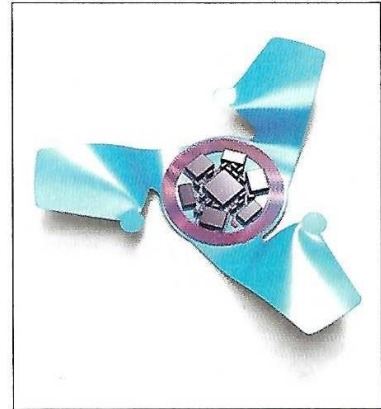
About the size of a grain of sand, the new flying microchip does not have a motor or engine. Instead, it catches flight on the wind and spins like a helicopter through the air toward the ground. (Image: Northwestern University)
