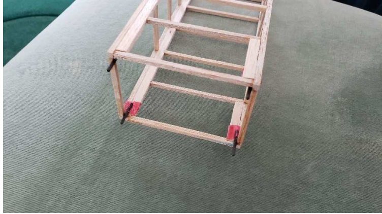
Carbon Fiber Rods that Align Fuselage Sections
