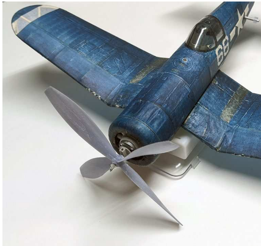
Peanut Hellcat with 3-D printed 4-bladed Prop
