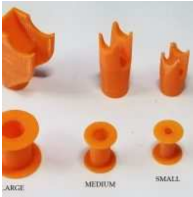
3-D Printed Stuffers and Bobbins
