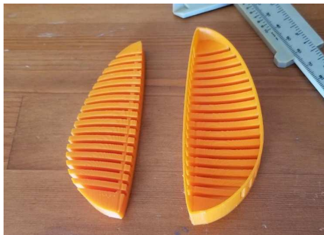
3-D Printed Mold Halves for Forming Helical Sheet Balsa Wood Propeller Blades
