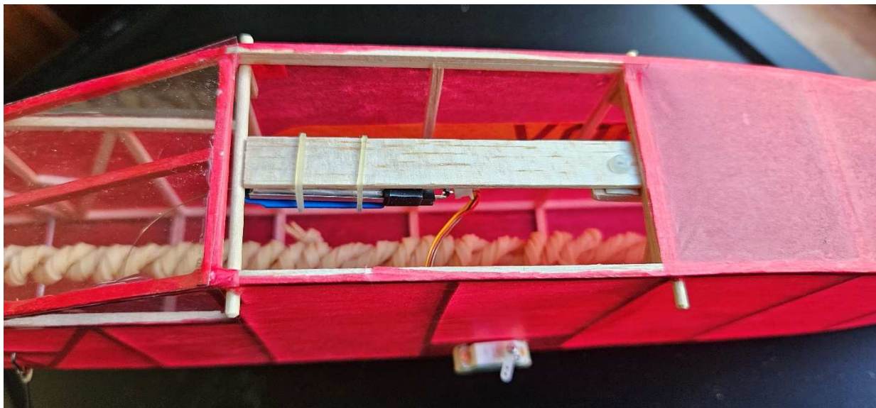
RF receiver and LiPo battery secured to mounting plank held to fuselage with plastic screw
