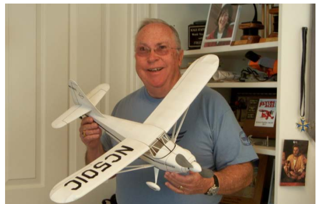
Roger Willis and his gorgeous new STINSON VOYAGER. Earl Stahl design from a Flyline kit. It has a 30" wing span and mounts a 9.5" prop with Gizmo Geezer, driven by 6 strands of 3/16th X 36". Weighs in at 80 gm.
