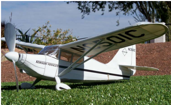
Roger Willis and his gorgeous new STINSON VOYAGER. Earl Stahl design from a Flyline kit. It has a 30" wing span and mounts a 9.5" prop with Gizmo Geezer, driven by 6 strands of 3/16th X 36". Weighs in at 80 gm.
