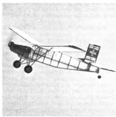
Here's Douglas Mooney's CO 2 Porter. He's almost as fine a builder at 15 as his dad. If flown with a Cox 010 with restrictor, additional dopping would be needed.
