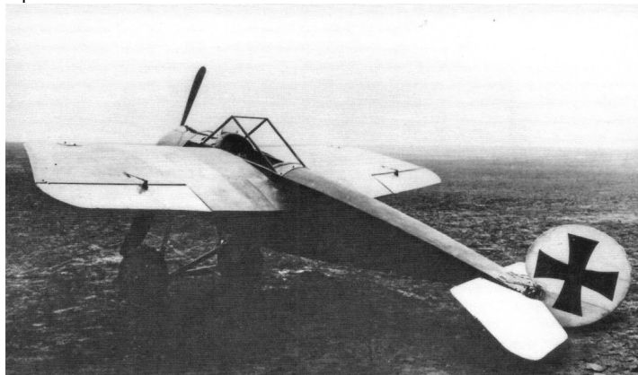
The diminutive Hergt Monoplane. Ailerons were fitted instead of wing warping. Surprisingly given its configuration and power, it appeared in August 1918.
