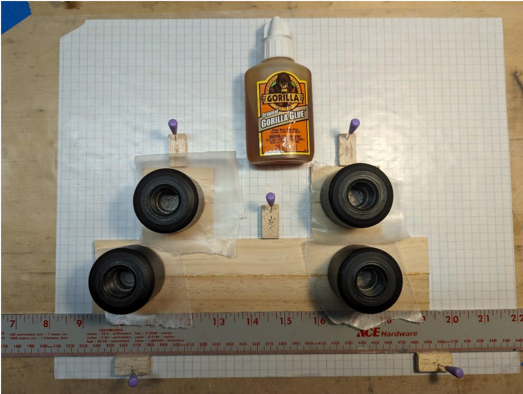
Brace parts together with pin blocks and a straight edge for strong and gap free glue joints.
