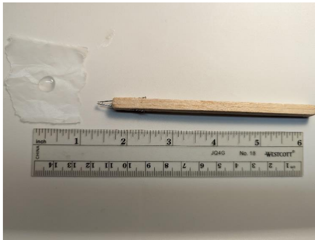
Figures 1-2: Simple glue tool; 1/4" sq x 4.5" balsa with pins. Correct size glue drop picked up by capillary action.
