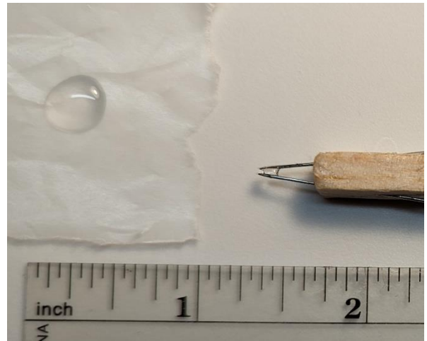
Figures 1-2: Simple glue tool; 1/4" sq x 4.5" balsa with pins. Correct size glue drop picked up by capillary action.
