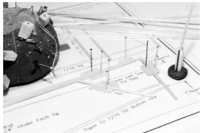
Rudder construction under way. Wedges used again to hold pieces in place. Drinking straw glue "well" at right.
