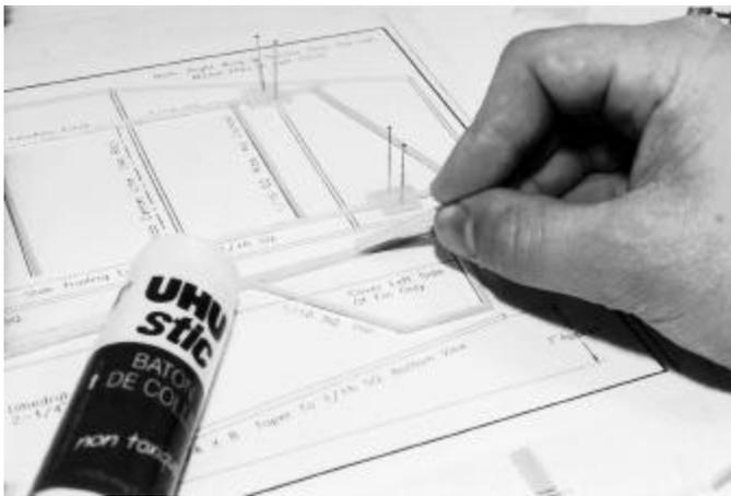
Glue stick can be used to apply adhesive to structure for covering. Soft balsa applicator makes job easier.
