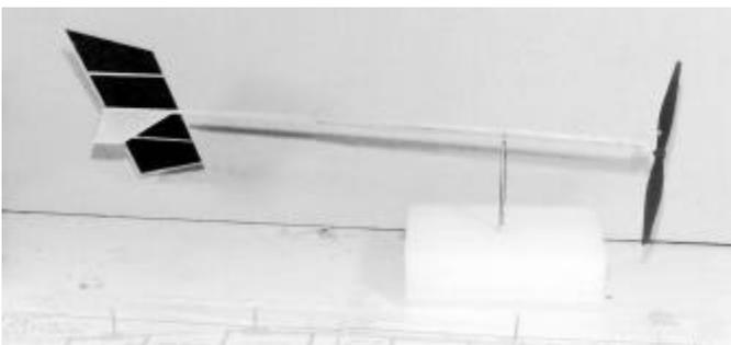
Completed motorstick and tail assembly is balanced to find proper horizontal Center of Gravity location. Though not shown here in this picture, the rubber motor (doubled to take up slack) should be attached for this procedure.
