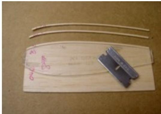
**Template for cutting sliced ribs. Make one from compact disc packaging plastic. Each slice produces a new rib.**
