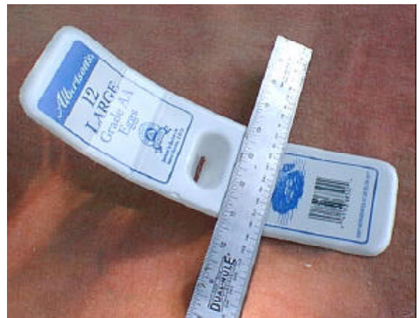
Figure 5. Use the ruler as a guide to bend dihedral into the wing (the model will not fly without it). Do this twice on each half of the wing. Note: If the foam cracks on the underside, rub Elmer's glue into the cracks and let dry.
