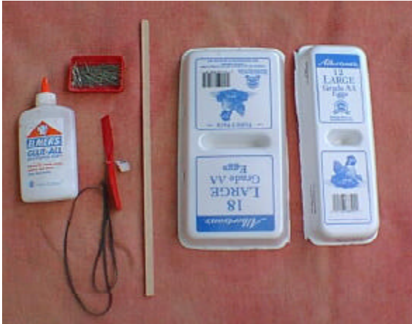
Figure 1. The materials that comprise the model are: Tops from a 12 egg and a 18 egg carton; a piece of 3/8" x 3/16" balsa; a propeller assembly from a Testors "Strato Streak", a rubber band, pins and Elmer's Glue or two part epoxy (not shown). Note: Do not use super glue or model airplane glue as they will melt the foam.
