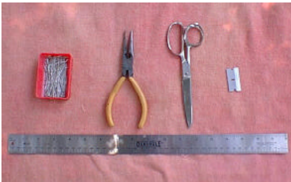
Figure 2. The tools used to build the model include pins, needle nose pliers, a scissors, a razor blade or exact knife, and a ruler. Note: Parents should make the cuts using the razor or knife.
