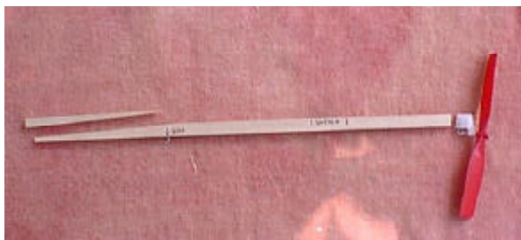
Figure 8. Cut the 3/8" x 3/16" balsa stick to 13 1/2" in length. Mark the location of the wing and the pin that will hold the rubber band on the side of the fuselage stick. Trim off excess wood behind the pin to save weight in the tail of the model. Note: Depending on the propeller assembly you use, small shims of balsa may be necessary to make the plastic fitting fit snugly over the front of the stick.
