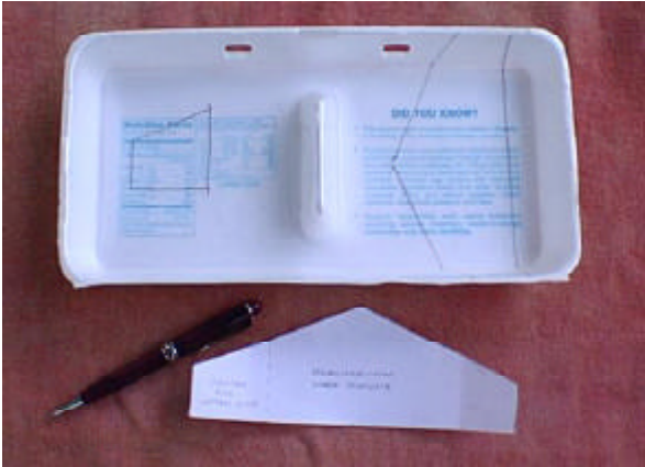
Figure 6. Cut the Stabilizer / fin template from the plan and trace it onto the inside of the 18 egg carton top using a pen or pencil.
