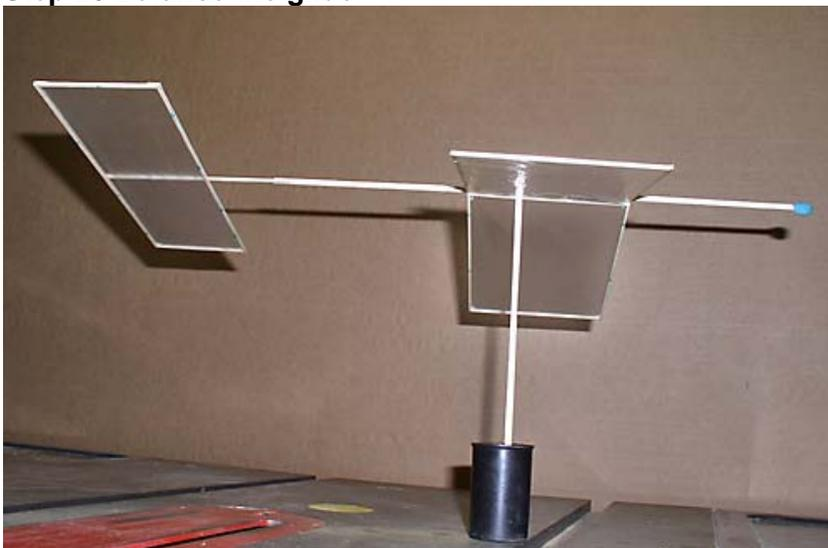
Balance the glider at the position shown on the plans by adding clay to the front of the glider (fuselage nose).
