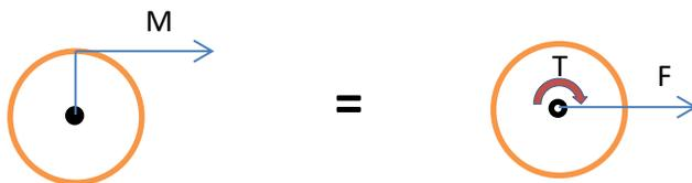
If the moments are not balanced, just like forces, the object will rotate about the pivot point. Thus, on an airplane, moments must be balanced as well.
