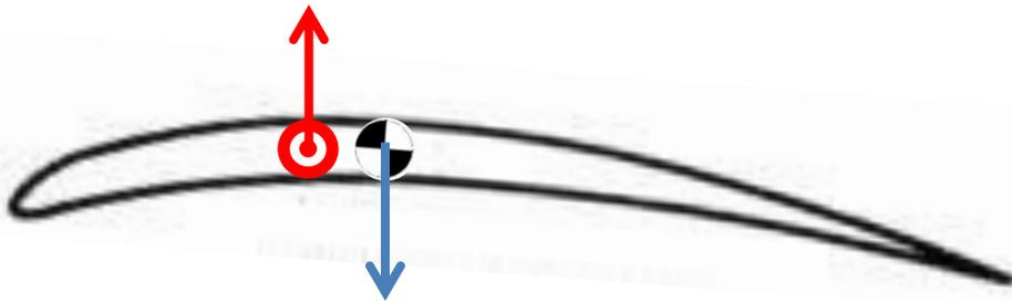
As we increase the angle of attack, the lift increases, but the gravity stays the same:
