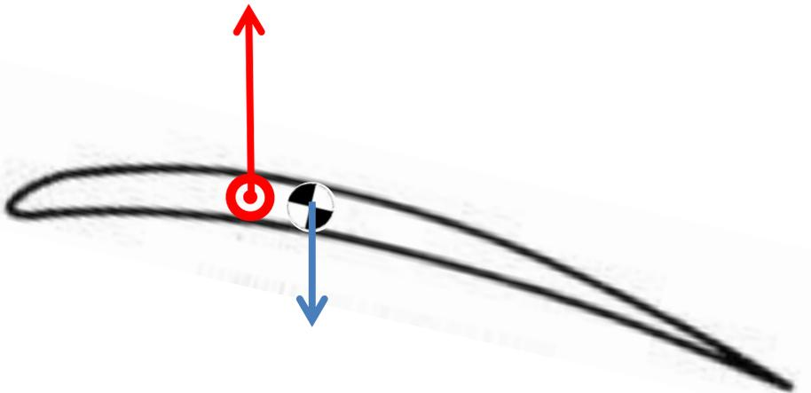
In this case, the moment about the CG due to lift increases in the clockwise direction, and so the plane wants to pitch up even more.
