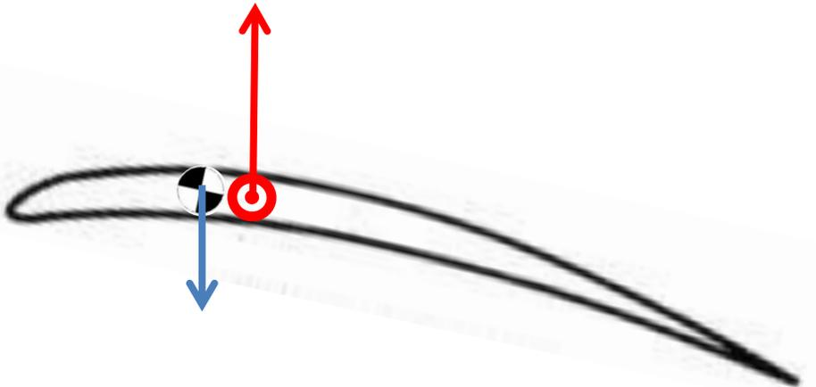
This increases the moment about the CG in the CCW direction, forcing the wing to reduce angle of attack! This is stable, as disturbances are cancelled.
