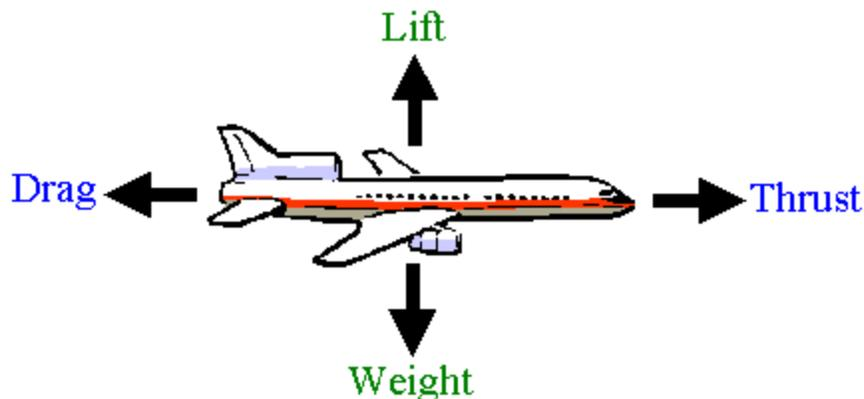
1. Weight is the force of gravity. It acts in a downward direction—toward the center of the Earth.
