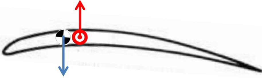
Now we slightly increase the angle of attack, which increases the lift at the CP (NP):
