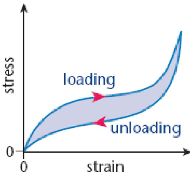
In this diagram, “strain” means stretching. In our case, while we stretch the rubber to aid in winding, the strain is caused by twisting the rubber. If you follow the “loading” curve, you see the rubber does not resist much at all in the beginning, then has a long period of accepting winds, or energy, and finally sharply increases in stress. If you kept adding energy after the sudden increase, the rubber breaks.
